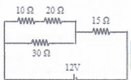
8 Calculate the the total current I, total voltage V and V<sub>2</sub>. R<sub>T</sub> = 2Ω
