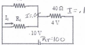
15 Use the diagram to calculate a) the total resistance in the circuit, b) the total current through the circuit, c) the total power the circuit consume, and d) the current through R<sub>2</sub>. (where R<sub>1</sub> = 10Ω, R<sub>2</sub> = 30Ω, R<sub>3</sub> = 30Ω, R<sub>4</sub> = 15Ω, V = 12V)
