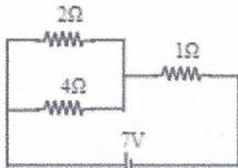
9 Calculate the equivalent resistance R and the total current I
