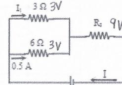
12 Calculate the the total current I and total voltage V.
