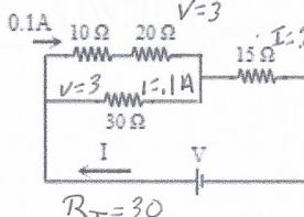
13 Calculate the the total current I and total voltage V.
