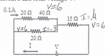
14 If R<sub>1</sub> = R<sub>2</sub>, calculate the R<sub>1</sub>, I<sub>1</sub>, and the total current I.
